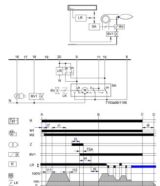
Load control with modulating controller with galvanically separated control contacts for positioning directions «OPEN» and «CLOSE».
